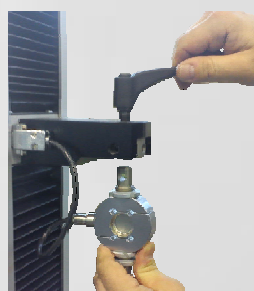
Easy load cell exchange Auto recognized
